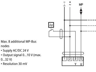
Max. 8 additional MP-Bus nodes • Switching current 16 mA @ 24 ٧
