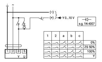
Override control with AC 24 V with Control remotely 0...100% with rotary switch
