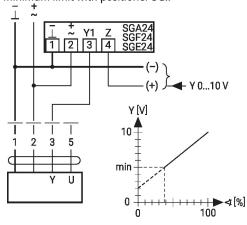
Override control with AC 24 V with Control remotely 0...100% with rotary switch
