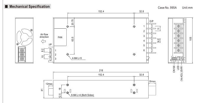
AC Input Terminal Pin No. Assignment
