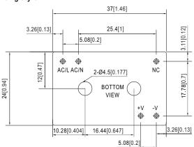
Case No.IRM03 Unit:mm[inch] Tolerance:±0.5[±0.02] unless otherwise specified
