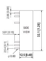
NOTE: Pin tolerance ±0.5mm
