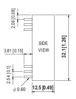
NOTE: Pin tolerance ±0.5mm
