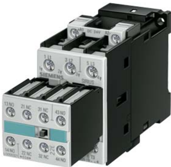
CONTACTOR, AC-3 5.5 KW/400 V, AC 230 V, 50 HZ, 3-POLE, 2 NO + 2 NC, SIZE S0, SCREW CONNECTION
