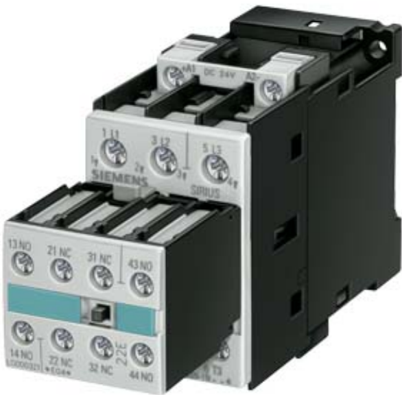
CONTACTOR, AC-3 7.5 KW/400 V, DC 24 V, 3-POLE, 2 NO + 2 NC, SIZE S0, SCREW CONNECTION
