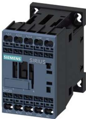
power contactor, AC-3e/AC-3, 7 A, 3 kW / 400 V, 3-pole, 230 V AC, 50/60 Hz,
