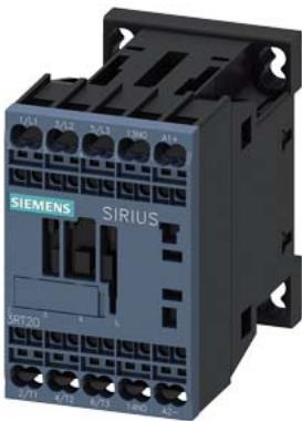
power contactor, AC-3e/AC-3, 12 A, 5.5 kW / 400 V, 3-pole, 24 V DC, auxiliary contacts: 1 NO, spring-loaded terminal, size: S00
