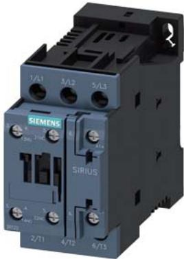
power contactor, AC-3e/AC-3, 12 A, 5.5 kW / 400 V, 3-pole, 110 V DC, auxiliary contacts: 1 NO + 1 NC, screw terminal, size: S0
