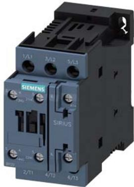
power contactor, AC-3e/AC-3, 32 A, 15 kW / 400 V, 3-pole, 24 V DC, auxiliary contacts: 1 NO + 1 NC, screw terminal, size: S0
