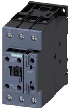
power contactor, AC-3e/AC-3, 80 A, 37 kW / 400 V, 3-pole, 230 V AC, 50 Hz,
