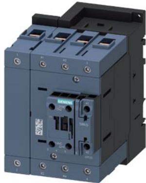
power contactor, AC-3, 80 A, 37 kW / 400 V, 4-pole, 230 V AC, 50 Hz, main contacts: 2 NO + 2 NC, auxiliary contacts: 1 NO + 1 NC, screw terminal, size: S3
