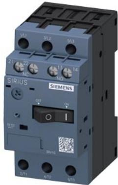
Circuit breaker size S00 for motor protection, CLASS 10 A-release 0.7...1 A N-release 13 A Screw terminal Standard switching capacity with transverse auxiliary switch 1 NO+1 NC
