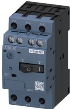
Circuit breaker size S00 for motor protection, CLASS 10 A-release 7...10 A N release 130 A Screw terminal Standard switching capacity with transverse auxiliary switch 1 NO+1 NC
