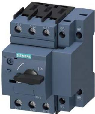
Circuit breaker size S00 for motor protection, CLASS 10 with overload relay function A-release 7...10 A N release 130 A screw terminal Standard switching capacity
